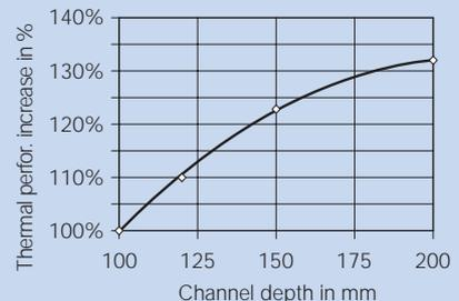
Tests carried out by the HLK Test Site of the University of Stuttgart with Meinertz ProLine Convection Grille type PL 07 05 0/5 at a temperature set of  $\Delta t$  42.5 K (70/55/20) °C, illustrated by the graph, show the influence of the channel depth on the thermal performance. This performance increase is dependent on the width of the convection grille.
