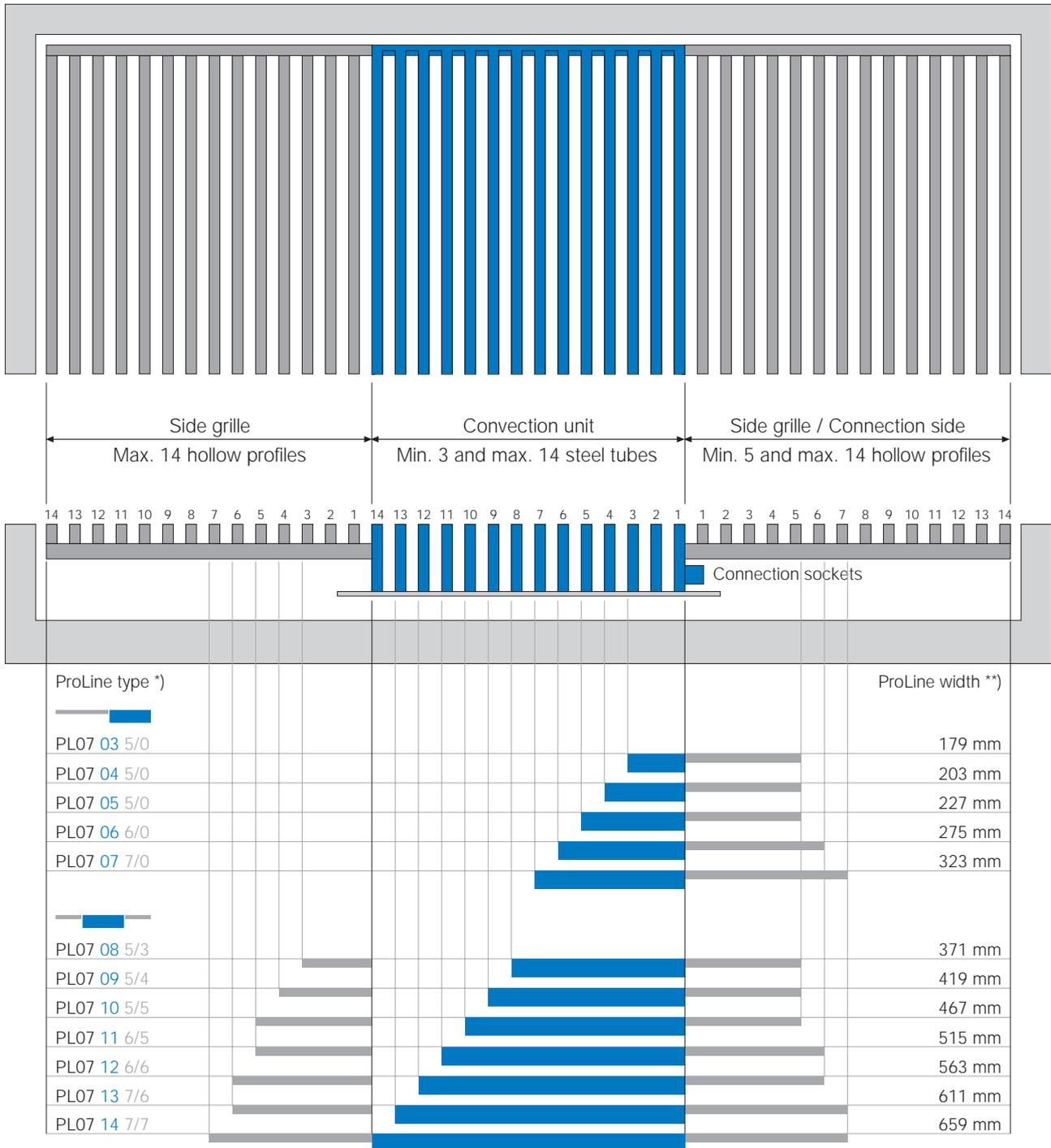
\*) The type designations indicate the minimum number of side grille profiles in relation to the number of convection tubes.
